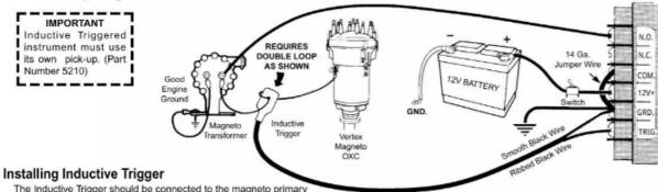
The Inductive Trigger should be connected to the magneto primary wire as shown here. Be sure to secure the Inductive Trigger with the nylon wire tie to prevent strain on magneto primary wires.
